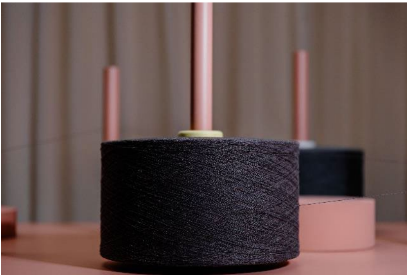
The WYRON truecycled® yarn consists of 50% post-consumer textile waste and 50% recycled polyester. Copyright: Brain of Materials
